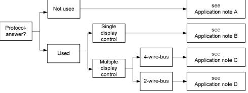
If the display should not send a protocol reply (normal case), application example A applies for activating one or more displays.
